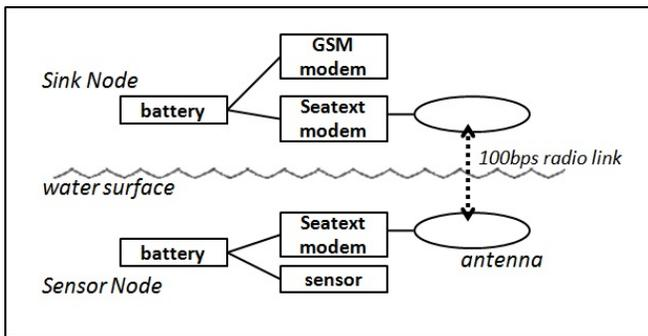
Fig. 2. Schematic of the sensor node and the sink
