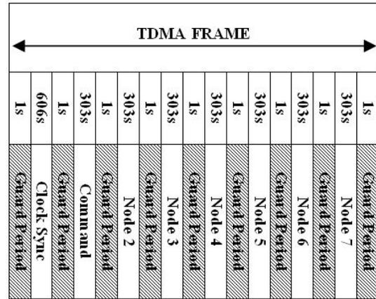
(b) Example TDMA Slot Configuration
