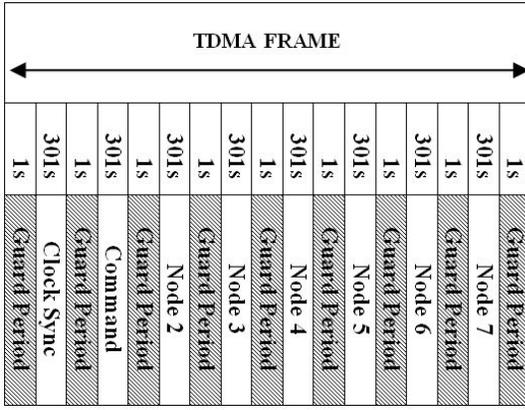
Fig. 3. TDMA Frame Structure
