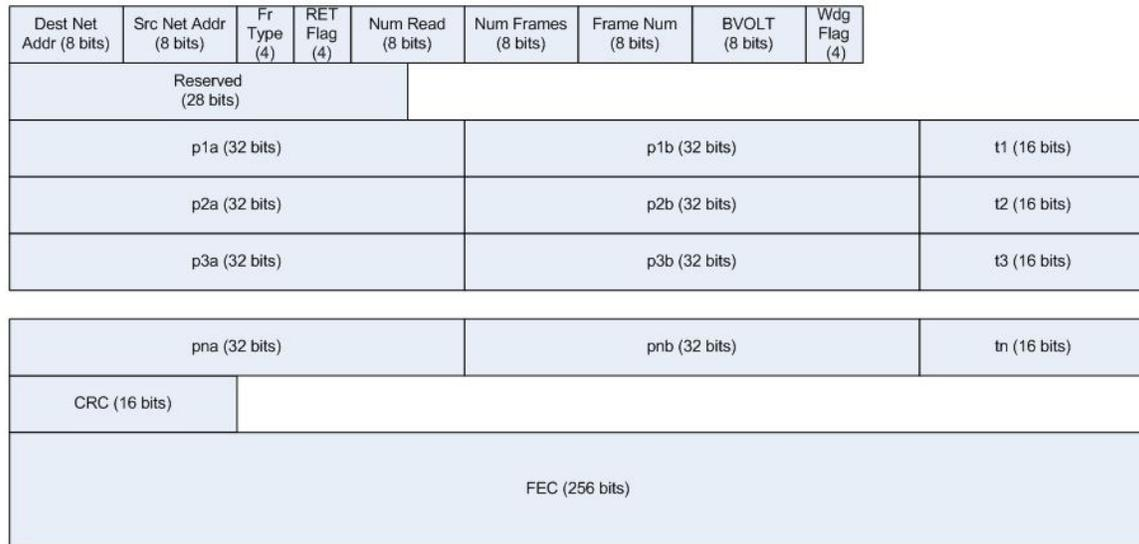
Fig. 5. Detailed Data Frame Structure
